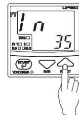
For example, to select thermocouple type J (°F), set the range code to 35.
