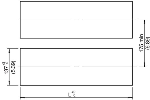
Side-by-side Mounting (vertically, max. 3 units)
