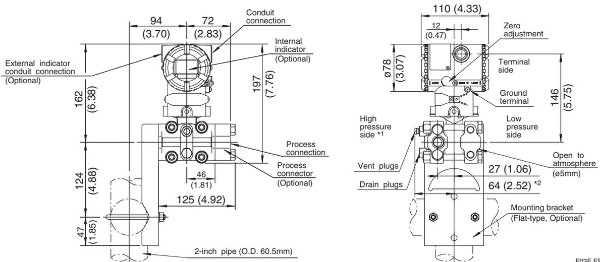
\*1: When Installation code 2, 3, or 8 is selected, high and low pressure side on above figure are reversed. (i.e. High pressure side is on the right side.)
