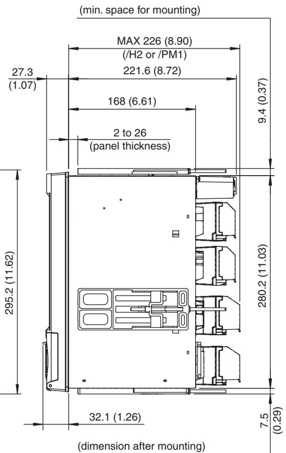
Note: If not specified, the tolerance is  $\pm 3\%$ . However, for dimensions less than 10mm, the tolerance is  $\pm 0.3\text{mm}$ .
